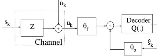
Fig. 1. Block diagram of a Wireless channel followed by a DFE.
