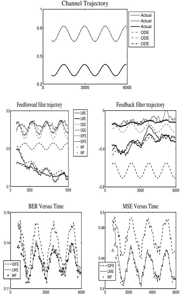
Fig. 4. A Stable channel with mean a constant multiple of  $[0.41, .82, .41]$ . It is obtained for  $f_d T = 0.001$ , i.e.,  $d_1 = 1.999982$ ,  $d_2 = -0.999947$  and  $\mu = 1.3997e - 010$ .
