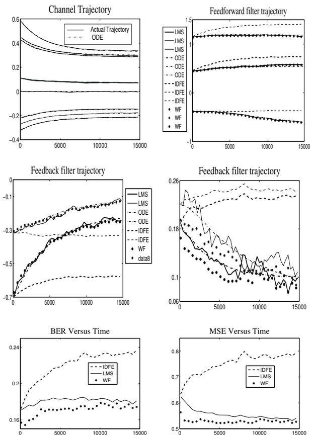
Fig. 2. A Stable channel with  $d_1 = 0.4995$ ,  $d_2 = 0.5$ ,  $\mu = 1e^{-4}$  and mean a constant multiple of  $[0.26, 0.34, 0.25, 0.064, -0.13, -0.19, -0.16, 0, 0.064, 0.064]$ .
